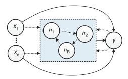
**FIGURE 3** Depiction of an RC architecture with one output. Fixed connections are shown as dashed lines, whilst trainable connections are shown as solid lines. The reservoir is highlighted with a light blue background.
